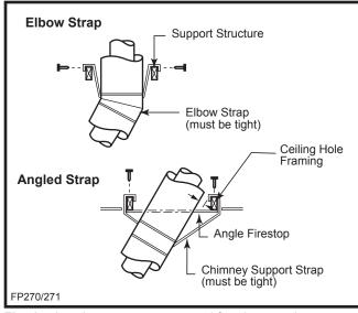
Fig. 17 Attach straps to a structural framing member.
